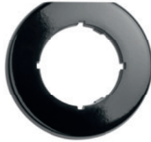
System covering external Ø 82 mm. For vertical and horizontal assembly. Suitable for all switches and outlets of the THPG switch system Bakelite. Product code 173092
